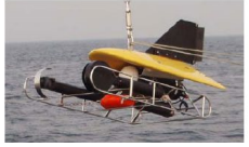
Fig. 2 Visual Plankton Recorder The device on the front right side (circular wheel) is a strobe, and the left one is a lens.
